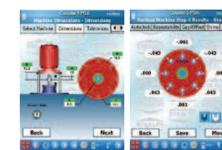
Vertical Motor Program: For vertically mounted, flange-type motors, enter motor dimensions, select tolerances and number of bolt holes and Couple5 will calculate the flange shim values.
