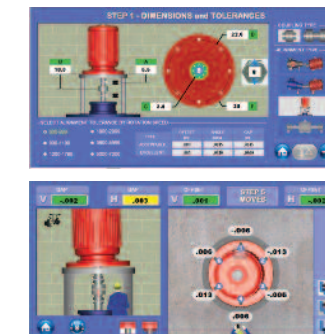
Vertical Motor Program: The industry's only vertical alignment display with live graphical displays of the motor's alignment along with shim values for all bolt-hole locations.
