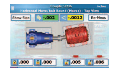
Bolt Bound™: Enter the pump's dimensions and then lock different combinations of the motor and pump feet to see how it affects the alignment. The graphics and shim values automatically update with each click.
