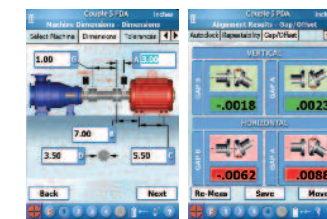
Spacer Shafts: Select Spacer Shafts, enter the spacer length and Couple5 will convert the alignment results to GapA/Gap B, the standard spacer-shaft format.
