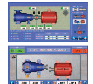
Bolt Bound™: Enter dimension of the pump, and then lock different combinations of the motor and pump feet to see how it affects the alignment. The graphics and shim values automatically update with each click.
