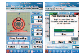
Taking Data with Uncoupled Shafts: Available on both Couple5 & 6, simply rotate laser to any position, then sweep the target past to take a data point. Continue until enough data has been taken to generate the results.
