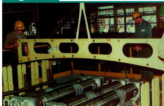
Originally segment rolls were aligned using templates and feeler gauges, introducing significant variability.
