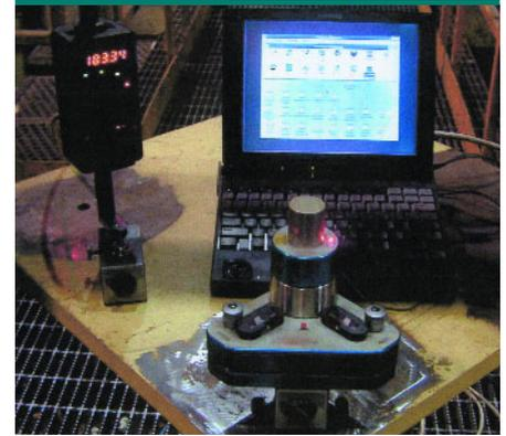
The laser alignment system is comprised of a single laser beam source, a height gauge target and software to calculate the shimming arrangement.
